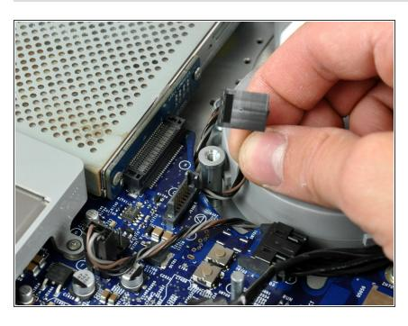
De-route the fan cable from around the edge of the logic board as necessary.
