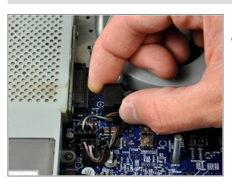
Disconnect the hard drive data cable connector from the logic board by pulling its connector straight up.
