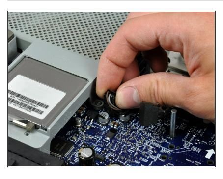
Disconnect the upper right fan cable connector from the logic board by pulling its connector straight up.
