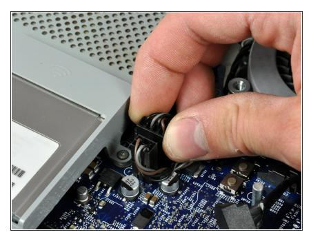
Disconnect the upper left fan cable connector from the logic board by pulling its connector straight up.
