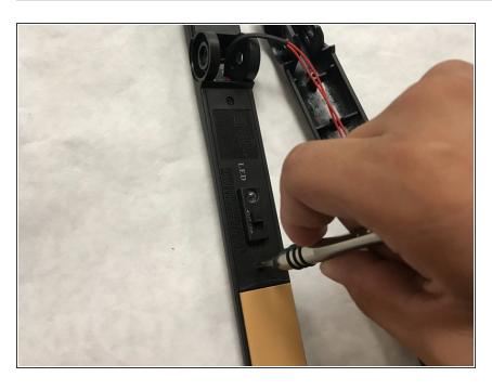
Remove the .53" long screw from the hinge pin.
