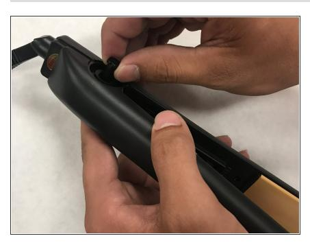
Remove the hinge pin.
