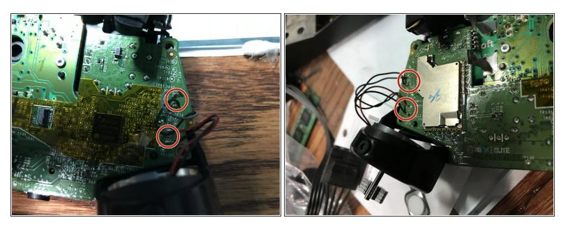
Desolder the 4 wires on each side, these control the vibrations and the RT LT
