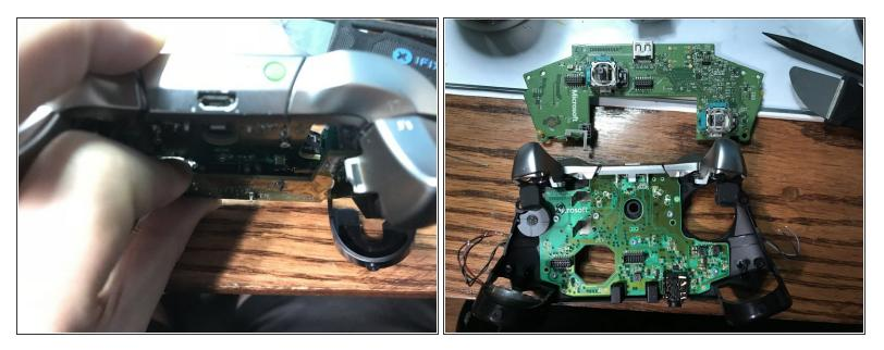
• Pull up from the "top" side of the controller on the sister board.
