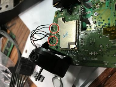
Desolder the 4 wires on each side, these control the vibrations and the RT LT
