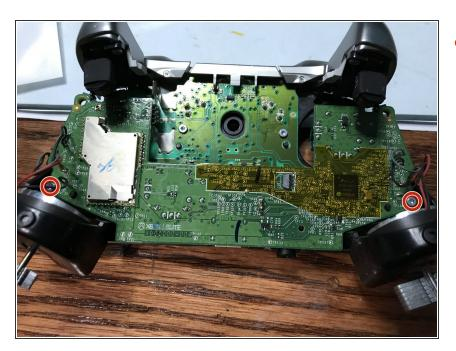
Remove the 2 Torx (T6) screws
