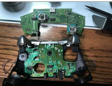
Pull up from the "top" side of the controller on the sister board.
