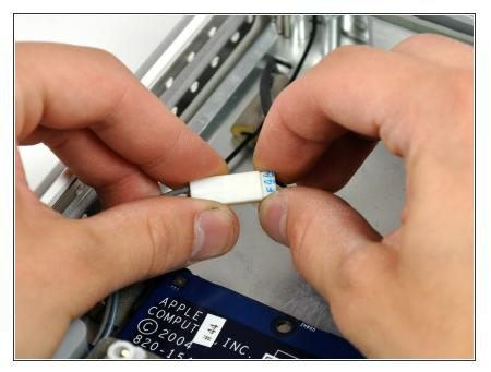
Disconnect the inverter-to-display cable connector by pulling it straight away from its socket.
