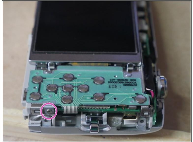
**⚠ Shock Hazard!** Do not touch anywhere along the top panel. Capacitor will still hold a residual charge that will shock you if touched. It is best to discharge the capacitor using the two metal solder joints on the top panel in front of the black tape
