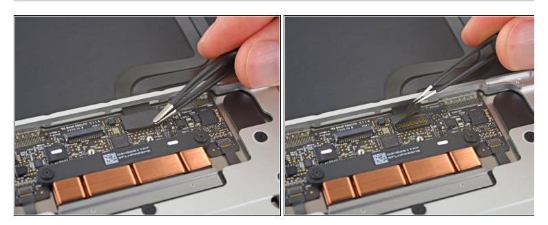
Use a pair of tweezers to remove the tape covering the keyboard ribbon cable connector on the trackpad.
