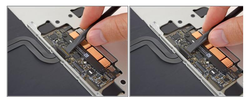
• Using a spudger, flip open the retaining flap on the keyboard ribbon cable ZIF connector.
