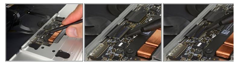
• Use a spudger to carefully flip up the retaining flap on the trackpad cable **ZIF** connector.
