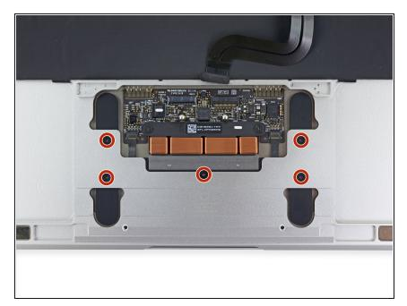
Remove the five 2.5 mm T3 Torx screws securing the trackpad to the case.
