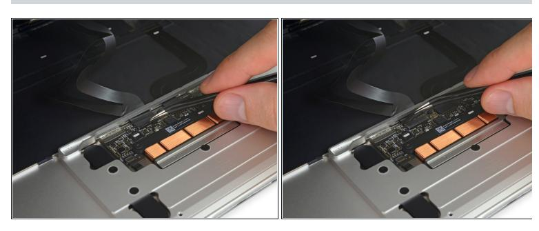
• Use tweezers to peel back the tape covering the trackpad cable ZIF connector.
