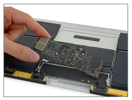
• Remove the logic board.
