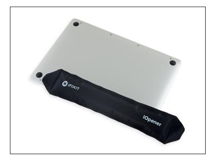
• <u>Prepare an iOpener</u> and heat the lower case directly beneath the right speaker for 1-2 minutes, in order to soften up the adhesive securing the speaker.
