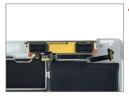
• Remove the two 4.1 mm T3 Torx screws securing the right speaker.
