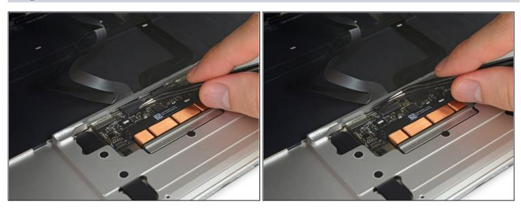
• Use <u>tweezers</u> to peel back the tape covering the trackpad cable ZIF connector.
