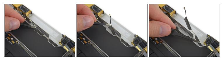
• Using tweezers, carefully peel up the tape securing the right antenna cable to the lower case.
