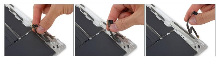
• Carefully peel away the audio board ribbon cable from the adhesive securing it to the lower case.
