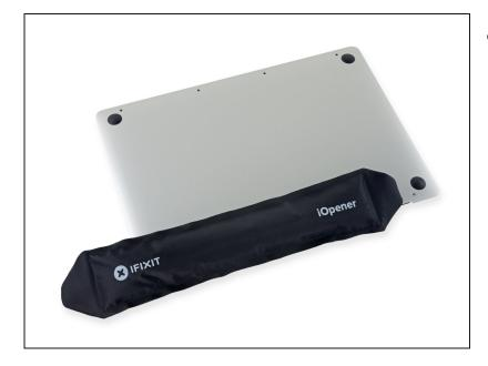
• <u>Prepare an iOpener</u> and heat the lower case directly beneath the left speaker, in order to soften up the adhesive securing the speaker.
