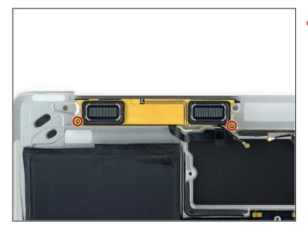
• Remove the two 4.1 mm T3 Torx screws securing the left speaker to the lower case.
