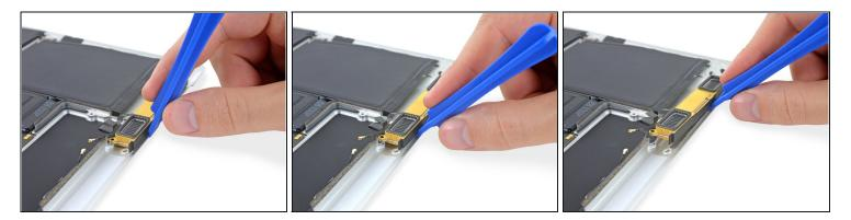
• Use a plastic opening tool to pry under the top edge of the left speaker, and separate it from the lower case.
