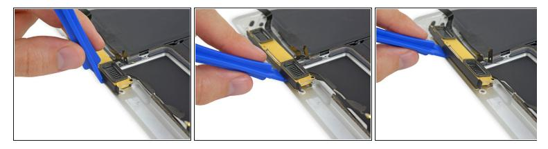
• Use a plastic opening tool to pry under the top edge of the right speaker, and separate it from the lower case.
