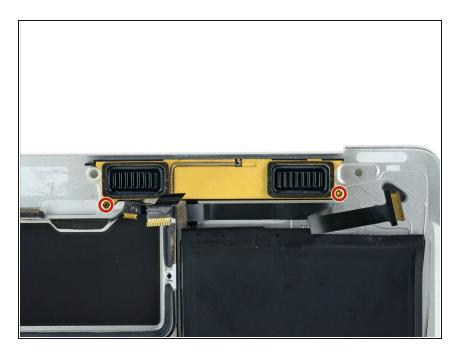
Remove the two 4.1 mm T3 Torx screws securing the right speaker.
