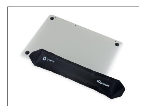
Prepare an iOpener and heat the lower case directly beneath the right speaker for 1-2 minutes, in order to soften up the adhesive securing the speaker.
