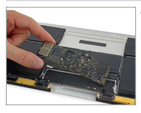
Remove the logic board.
