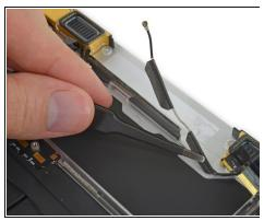
• Using tweezers, carefully peel up the tape securing the right antenna cable to the lower case.
