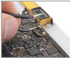
Pry up the second antenna connector to disconnect it.
