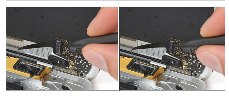
• Use a spudger to flip open the retaining flap on the audio jack board cable ZIF connector.
