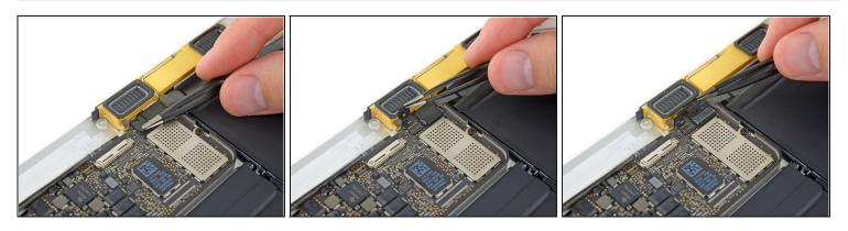
• Use <u>tweezers</u> to peel up the tape covering the two ZIF connectors—one for the right speaker cable, and one for the audio jack board cable.
