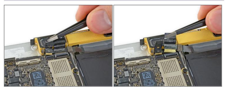
• Carefully pull straight back on the two pieces of tape you just peeled up to disconnect the two ribbon cables.
