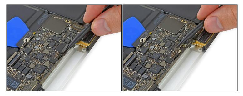
• Use the point of a spudger to peel up the foam pad covering the two antenna connectors.
