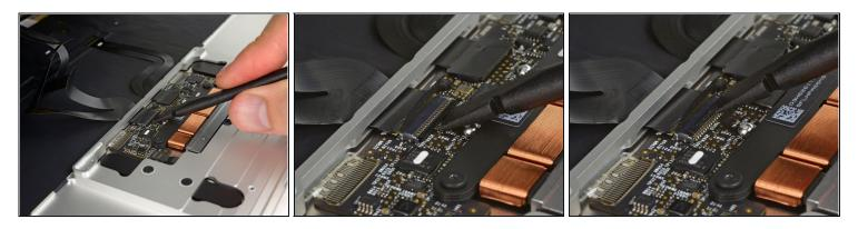
• Use a spudger to carefully flip up the retaining flap on the trackpad cable <u>ZIF</u> <u>connector</u>.
