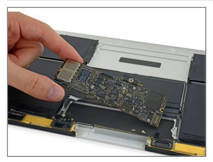
• Remove the logic board.
