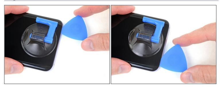
• Slide your opening pick along the lower edge of the display to separate the adhesive underneath.
