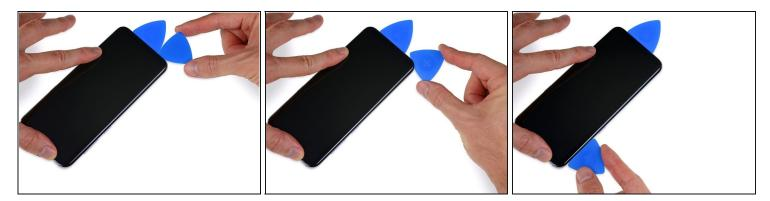
• Use your opening pick to separate the adhesive under the left side of the display.
