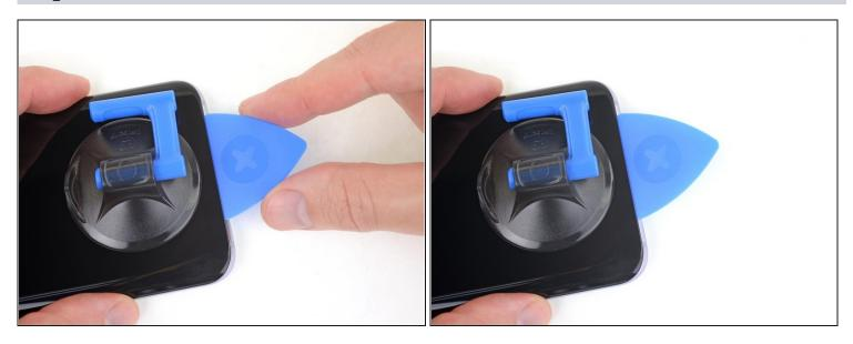
• Leave the pick in place and grab a second pick as you proceed to the next step. Leaving the pick inserted can help prevent the glue you just separated from re-adhering.
