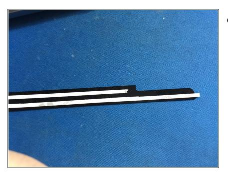
Put double-sided tape on the back of the new bezel.
