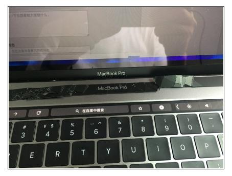
Install the bezel into its original position.
