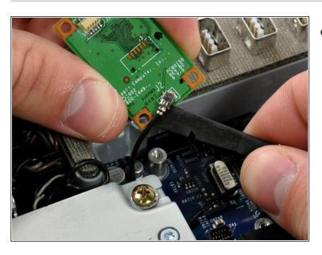
Use a spudger to pry the Bluetooth antenna connector up off the Bluetooth board.
