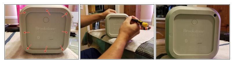
Use a thin flat screwdriver to pry these out.
