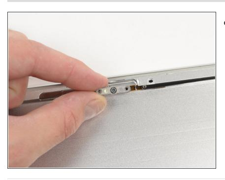
Lift and remove the camera assembly out of the rear display bezel.
