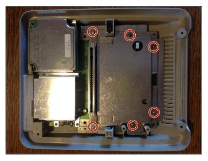
• The shield is held by 6 Philips #2 screws.
