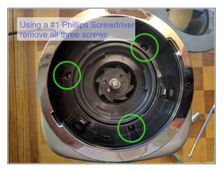
Using a #1 Phillips Screwdriver remove each of the three top screws and set them aside.
