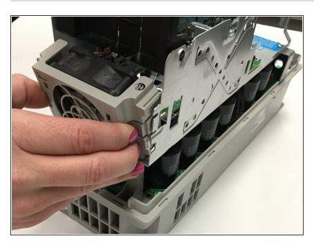
Remove the upper fan by pinching the tabs found on each side and pulling.
