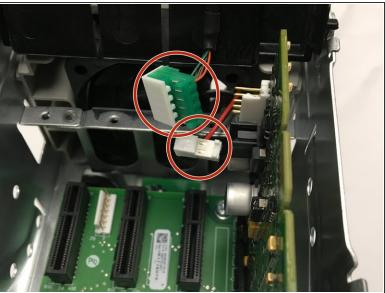
Remove the two connectors located at the top of the drive near the Keypad Panel by pulling them with two fingers. Be sure to pull on the plastic connectors and not on the wires.
