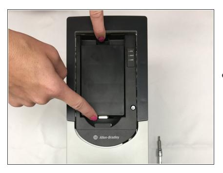
The PF755 will either have a cover plate, as shown in this guide, or a keypad. To remove these, press on
