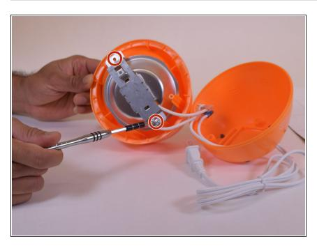
Remove the two screws from both sides of the heating coil.
