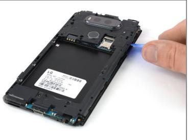
• Slide the opening pick along the mid frame and flip it sideways to open the plastic clamps holding the motherboard cover in its place.
