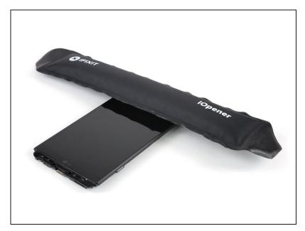
Use an iOpener to loosen the adhesive beneath the secondary rear facing camera.
