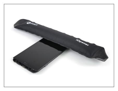
Use an iOpener to loosen the adhesive beneath the secondary rear facing camera.
