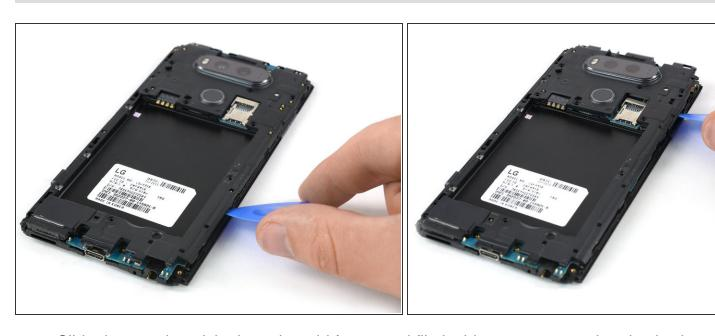
Slide the opening pick along the mid frame and flip it sideways to open the plastic clamps holding the motherboard cover in its place.
