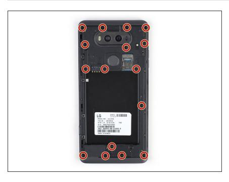
Remove the sixteen 4mm Phillips #00 screws attaching the back cover to the motherboard.
