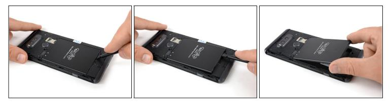
A Before disassembling your phone, discharge the battery below 25%. A charged lithiumion battery can catch fire and/or explode if accidentally punctured.
