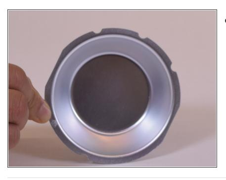
Remove the heating bowl from the plastic housing.
