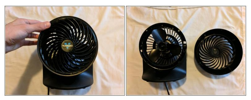
• Once the screws are removed, turn the fan back over. Use your hands to pull the front grill cover off.
