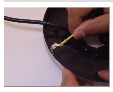
Detach the power cord's grounding wire (yellow with green stripes) from the edge. First unbend the silver strip, then pull upwards with a small jiggle.
