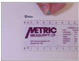
Remove the two rounded top (12mm) Phillips Head screws from the 1" bar holding down the power cord.
