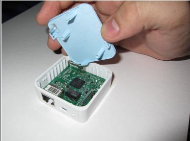
• Once the cover is loose, the cover can be removed, revealing the router's main circut board.
