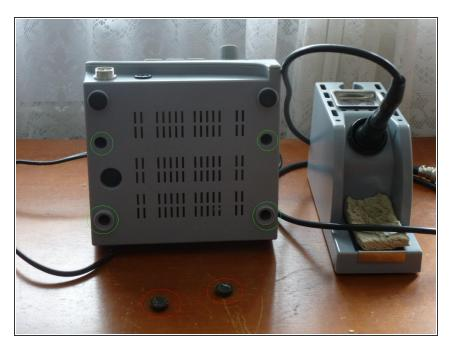
... by nails or by flat screwdriver and you will see the second pair of holes with screws.
