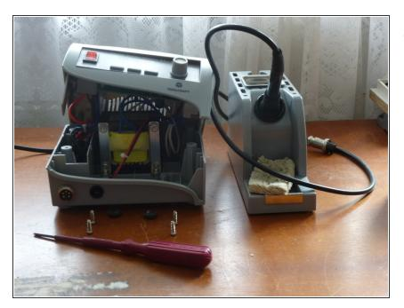
... by Phillips #1 screwdriver and you can open the body of the solder station.
