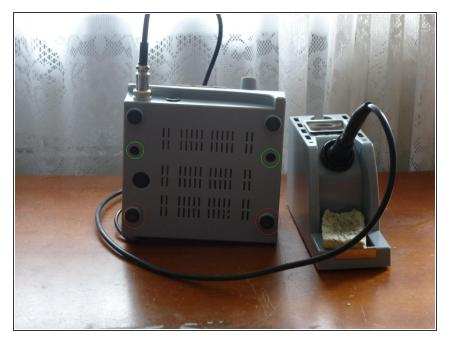
• There are two holes with screws on the bottom side (green circles on the picture) and the 2-nd pair of screws is under the two rubbery "legs" (red circles).
