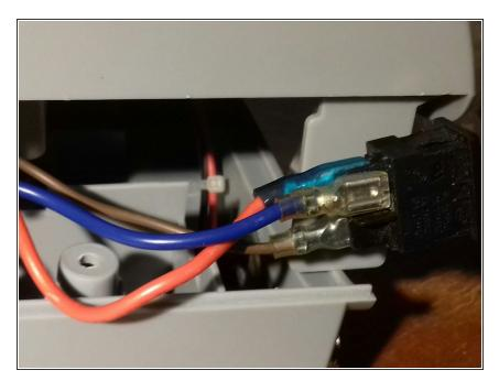
The cables connected to switch: ON is Up , from inside: 1) RED + BLUE
