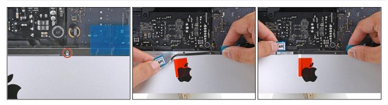
(i) The microphone hole is <u>the center hole</u> flanked by two larger holes.
