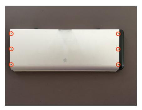
Start by removing the 6 3 mm Y00 screws from the top side of the battery
