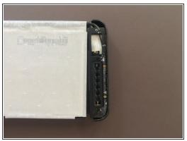
(i) When reassembling it's easier to attach the plastic cover onto the plastic bracket before inserting the pack back into the aluminium casing.
