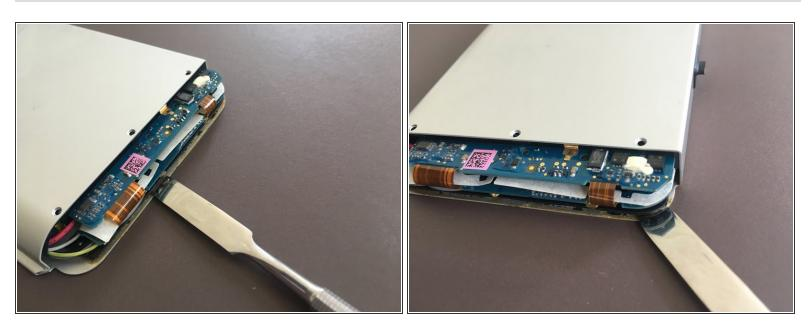
Work your way across the entire edge of the battery to free the plastic bracket from the aluminium casing.
