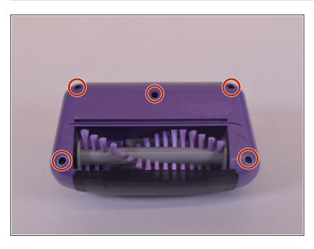
Use a Phillips #1 screwdriver to remove the five 14mm screws from the face of the motorized brush.
