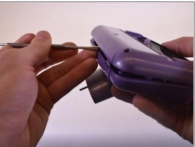
Separate the motorized brush face plate by using a flat prying tool.
