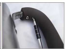
• Use a Phillips-Head (PH1) screwdriver to loosen the two screws that attach the handle to the pot.
