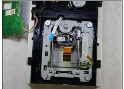
With the board freed from it's trappings, locate the pin securing the wires connected the board.
