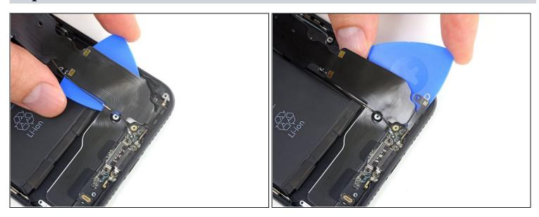
• Carefully slide your pick from the corner of the battery to the corner of the iPhone to separate the portion of the flex cable adhered to the outer frame.
