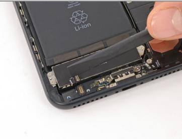
• Pry up the Taptic Engine's ribbon cable connector to disconnect it.
