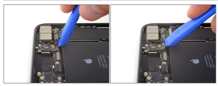
Use a fingernail or the sharp end of an iFixit opening tool to pry up and disconnect the antenna flex cable connector from the logic board.
