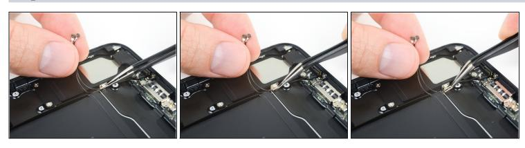
• Carefully de-route the two coaxial cables from the metal bracket holding them to the side of the speaker.
