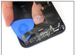
• Slide your pick across the width of the iPhone to separate all the remaining strands of the flex cable from the rear case.
