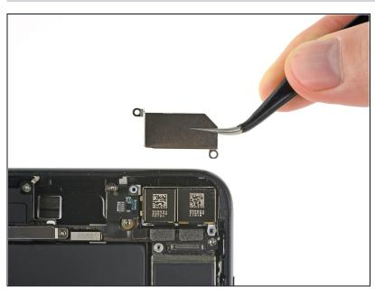
• Remove the bracket covering the rear-facing camera.
