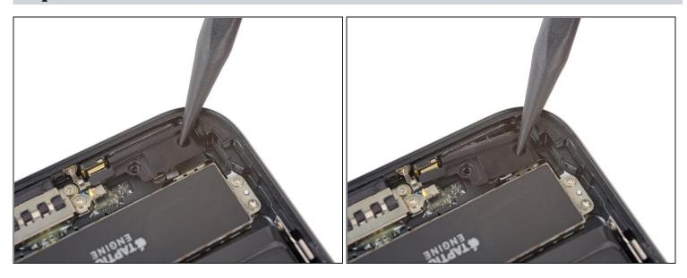
• Gently push the barometric vent in the direction of the Taptic Engine to separate the adhesive securing it to the bottom edge of the iPhone.
