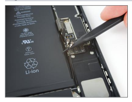
Use the point of a spudger to carefully de-route the two coaxial cables from the small metal clip holding them to the logic board.
