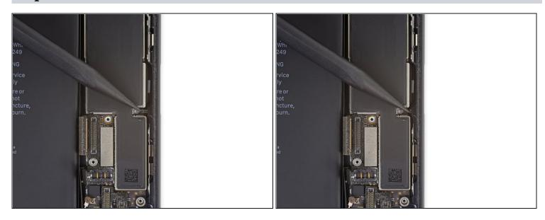
• Use the point of a spudger to push the SIM card eject plunger out of the logic board's way.
