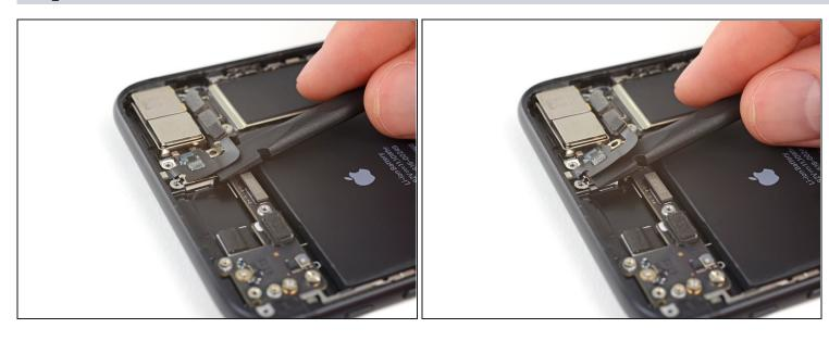
• Slide the flat edge of a spudger underneath the antenna flex cable to separate the adhesive holding it in place.
