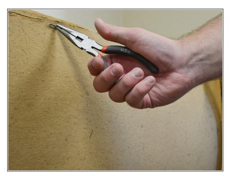
Using a pair of pliers, remove the existing staples from the bottom of the dresser.
