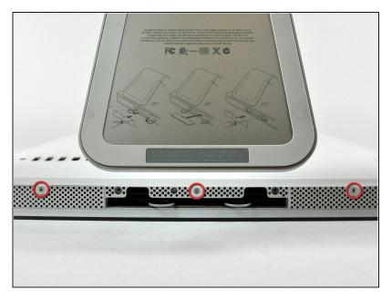
Remove the three T8 Torx screws securing the front bezel to the rear panel.
