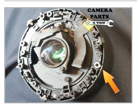
Next to your previous mark make a mark on the outer barrel to help with re-assembly.. That mark will line up with 0.25m lettering on the front barrel
