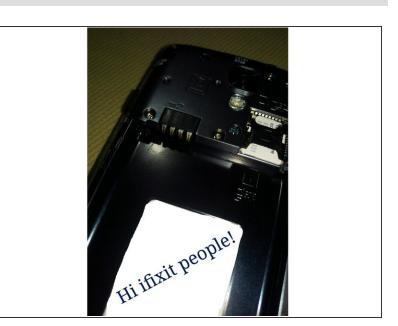
Note the location of the screws to remove the inner rear panel.
