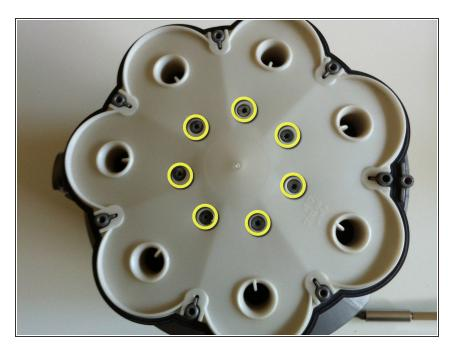
Remove the seven torx screws which hold the cyclone manifold in place. You need a torx T15 driver for this.
