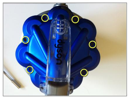
Remove the seven torx screws which hold the top cover in place (one is located in the middle of the handle). You need a torx T15 driver for this.
