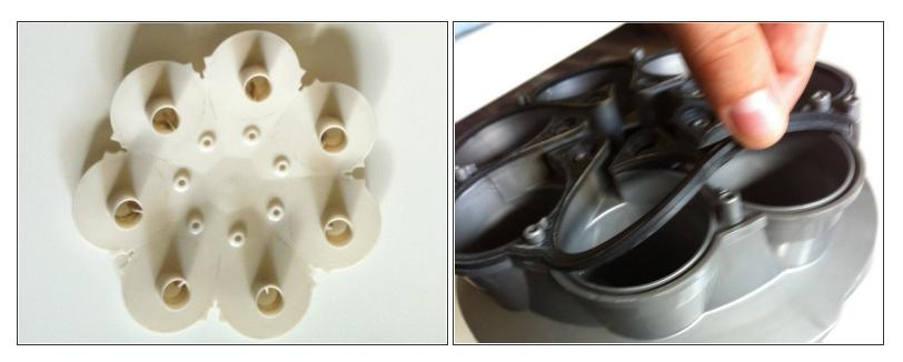
• Remove the manifold and the gasket underneath it.
