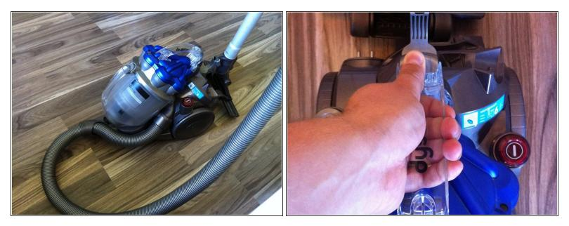
• Detatch the cyclone assembly from the main unit.
