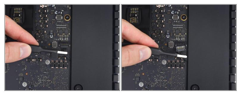
Gently pull the right speaker cable connector straight down and out of its socket on the logic board.
