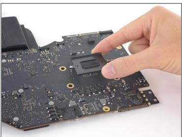
• Lift the heat sink retaining spring and its bracket off the logic board.
