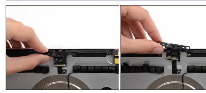
Lift and remove the camera assembly from the iMac.
