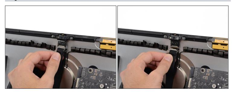
• Gently pull the camera cable straight down from its socket on the camera board.
