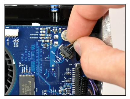
• Disconnect the optical drive fan cable connector from the logic board by pulling it straight away from its socket.
