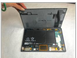
Remove the back cover by lifting up one corner using the plastic opening tool, and then removing the adhesive around the cover.
