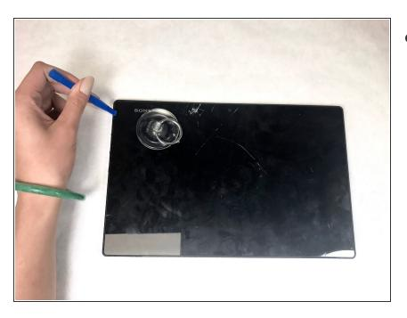
Gently pry the edge of the screen working around while heating.
