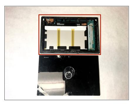
Clean adhesive from perimeter of frame to prepare for new screen.
