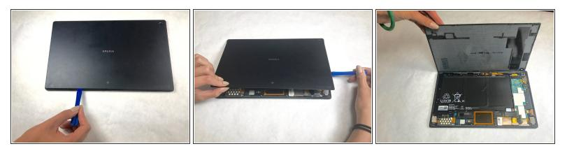
• Remove the back cover by using the plastic opening tools.
