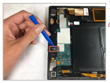
Slide the ribbon cable out of motherboard.
