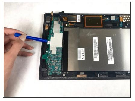
Remove the motherboard by gently prying up. Once it is loosened from the adhesive you may need to slide it away from the battery while lifting.
