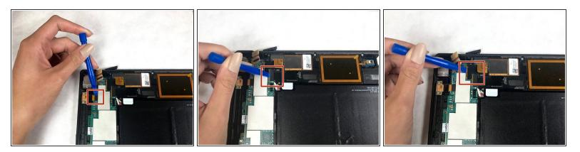
• Disconnect the 3 ribbon cable connectors from the mother board near the USB port and speaker.
