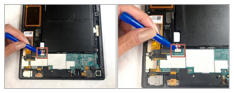
Disconnect the battery by lifting the connector straight up from the motherboard with a plastic opening tool or equivalent.
