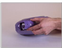
Locate and remove the 7.5mm Philips screw holding the battery cover in place on bottom of the vacuum.
