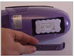
Once the cover is removed, slide the plastic retaining bracket down and pull out to remove.
