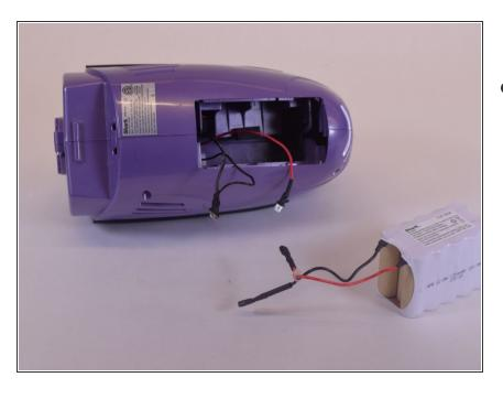
Completely remove the old battery from the vacuum. To reassemble your device, follow these instructions in reverse order.
