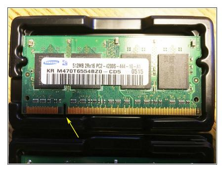
Gently insert the new memory modules into the slots where you removed the old memory. Note the slot in each module, which prevents you from inserting the memory module in the wrong orientation.
