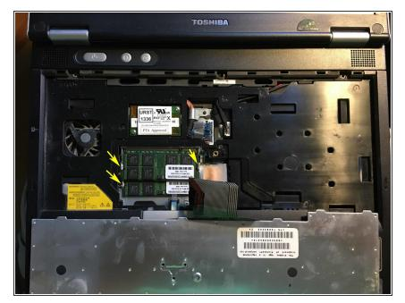
To remove a memory module, gently slide the module's retaining clips toward the outside edges of the laptop. In the photo one of the retaining clips is hidden underneath the keyboard ribbon cable.
