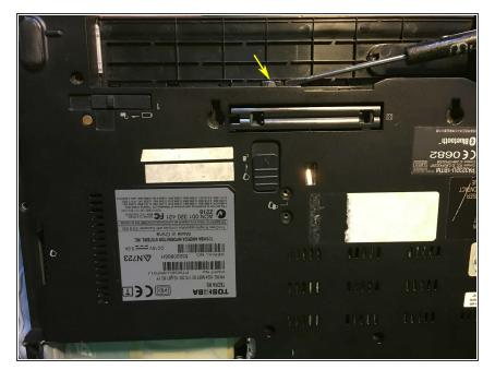
Once the battery is out, you have access to a small retaining screw at the bottom of the battery compartment. Remove this screw.
