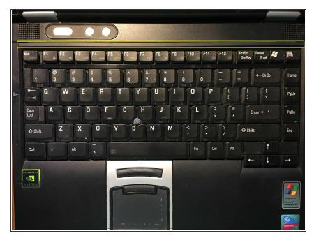
Turn the laptop right side up and open the lid. Carefully pry off the plastic keyboard trim (outlined in yellow). It comes off very easily once you remove the retaining screw (step 2).
