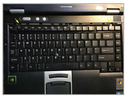
Remove the two screws at the top of the keyboard. After removing the screws, carefully slide the keyboard forward until the plastic fingers on its lower edge are free of the case. Then flip the keyboard toward you, taking care not to damage the ribbon cable connecting it to the laptop.
