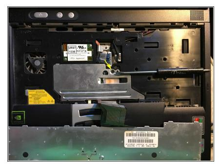
A single screw holds a sheet metal memory access cover in place.
