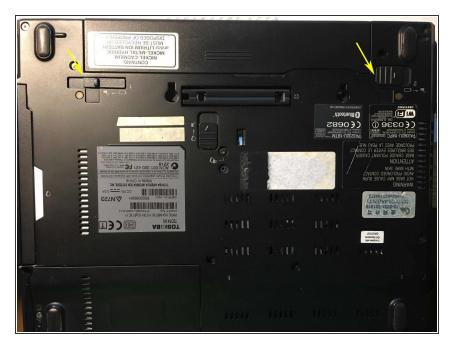
Turn the laptop upside down, with the battery at the upper edge. While sliding the battery latches, push the battery away from you to slide it out of the laptop.
