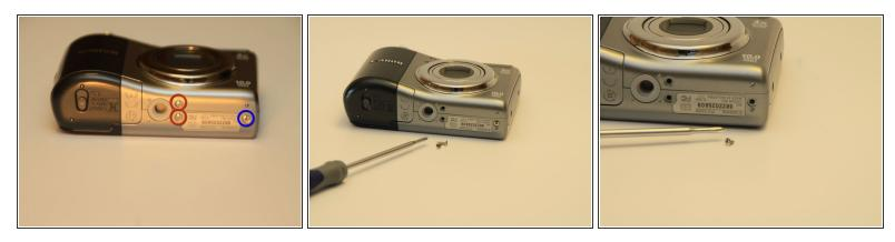
Remove the two coarse thread screws and the single fine thread screw from bottom the camera.
