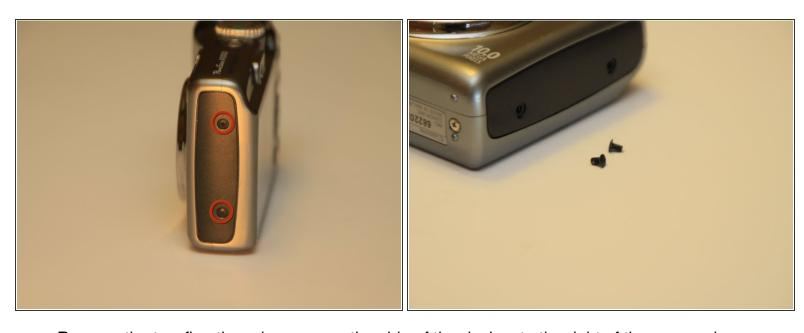
Remove the two fine thread screws on the side of the device, to the right of the camera lens.
