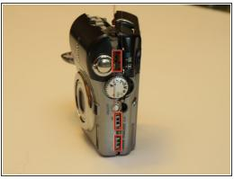
Gently pry apart the two covers starting from the bottom. When there is a 1/4" gap, run your finger gently along the top of the camera, on the back cover, to release the three catches that secure the shell.
