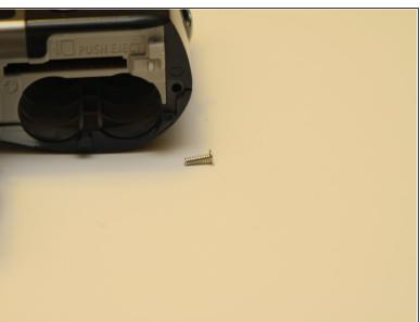
Remove the one coarse thread screw underneath the battery cover.
