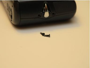
Remove the two coarse thread screws on the side of the device, to the left of the camera lens.
