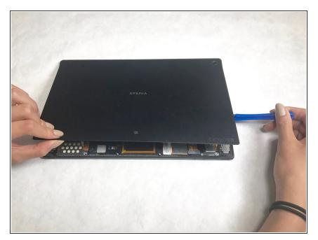
Slide the plastic opening tool along the edge of the device removing the adhesive.
