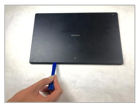
• Place the plastic opening tool in the corner of the device.
