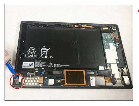
Using the plastic opening tool, gently lift the speaker out of place.
