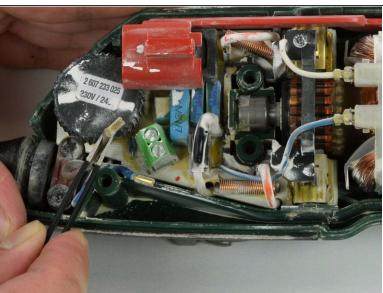
Pull the wires out of the holder with a gripping tool. For example, with a pair of <u>tweezers</u> or a small, flat pair of pliers.
