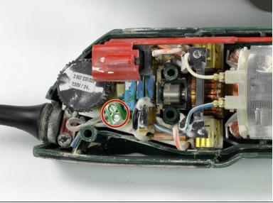
Now first loosen the two slotted screws # 3 so that the wires can be pulled out of the clamp.
