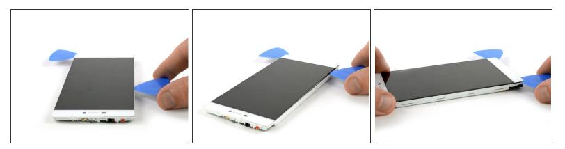
Insert just the tip of the opening pick and slide it along the left side of the phone to separate the display from the frame.
