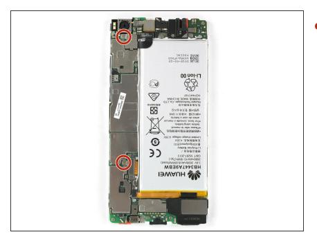
Remove the two Phillips #00 that hold down the two metal clamps covering the front camera, the display and battery flex connectors.
