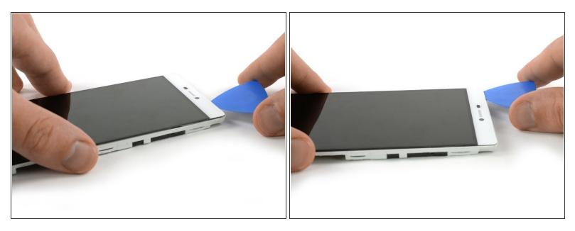
Insert another opening pick at the top of the phone and loosen the adhesive under the upper part of the display.
